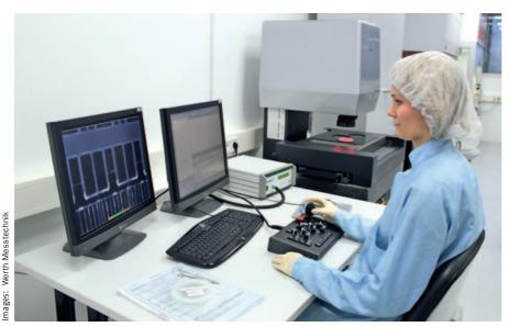
Figure 1. In the clean room: Employees use a 3D CNC multisensor coordinate measuring machine with a chromatic focus sensor for measuring wafer thickness.
