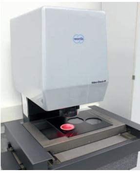
Figure 3. Scanning: Wafers are inspected for particulate impurities using the image processing sensor.
