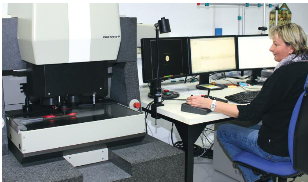
Fig. 1. The fixed portal measuring machine is equipped with telecentric optics as well as a fiber probe and a conventional trigger probe.
