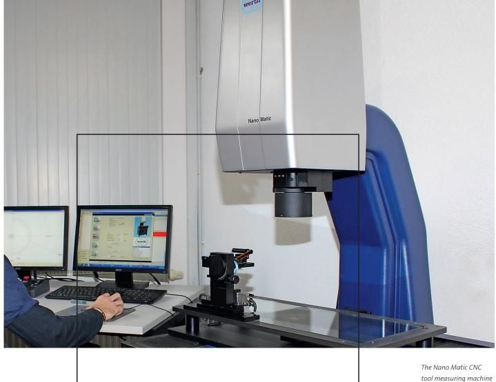
tools fall into after the production process. If we offer a ball-nose mill with a form accuracy of  $\pm$  3 micrometers over the entire contour, then this will also be shipped to the customer in that condition — exclusively at the A quality level."
