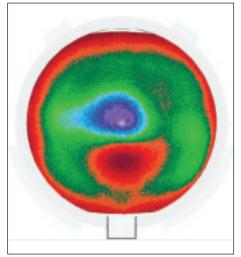
An LED lens before (left) and after tool correction - colour coding identifies errors
