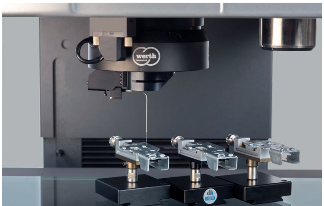
Figure 1. Multisensor measurement using a fiber probe, image processing sensor, and chromatic focus point sensor; – the fiber probe is placed in front of the beam path of the image processing sensor with zero offset. (© Werth)
